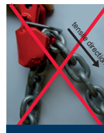
Incorrectly attached chain
