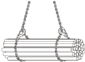
Figure 12: Reverse choke hitch
